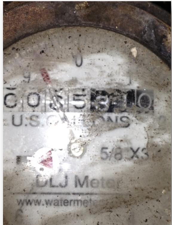
Figure 9. Two water meters purchased and installed on March 20 th , 2014 to measure pen wash down water additions to manure volume. Meters readings were 96,609.6 and 65,319.3 gallons for meter 1 and 2 on September 10 th , 2014.
