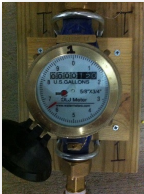
Figure 8. Two water meters purchased and installed on March 20 th , 2014 to measure pen wash down water additions to manure volume. Initial meters readings were 126.6 and 80.2 gallons for meter 1 and 2.
